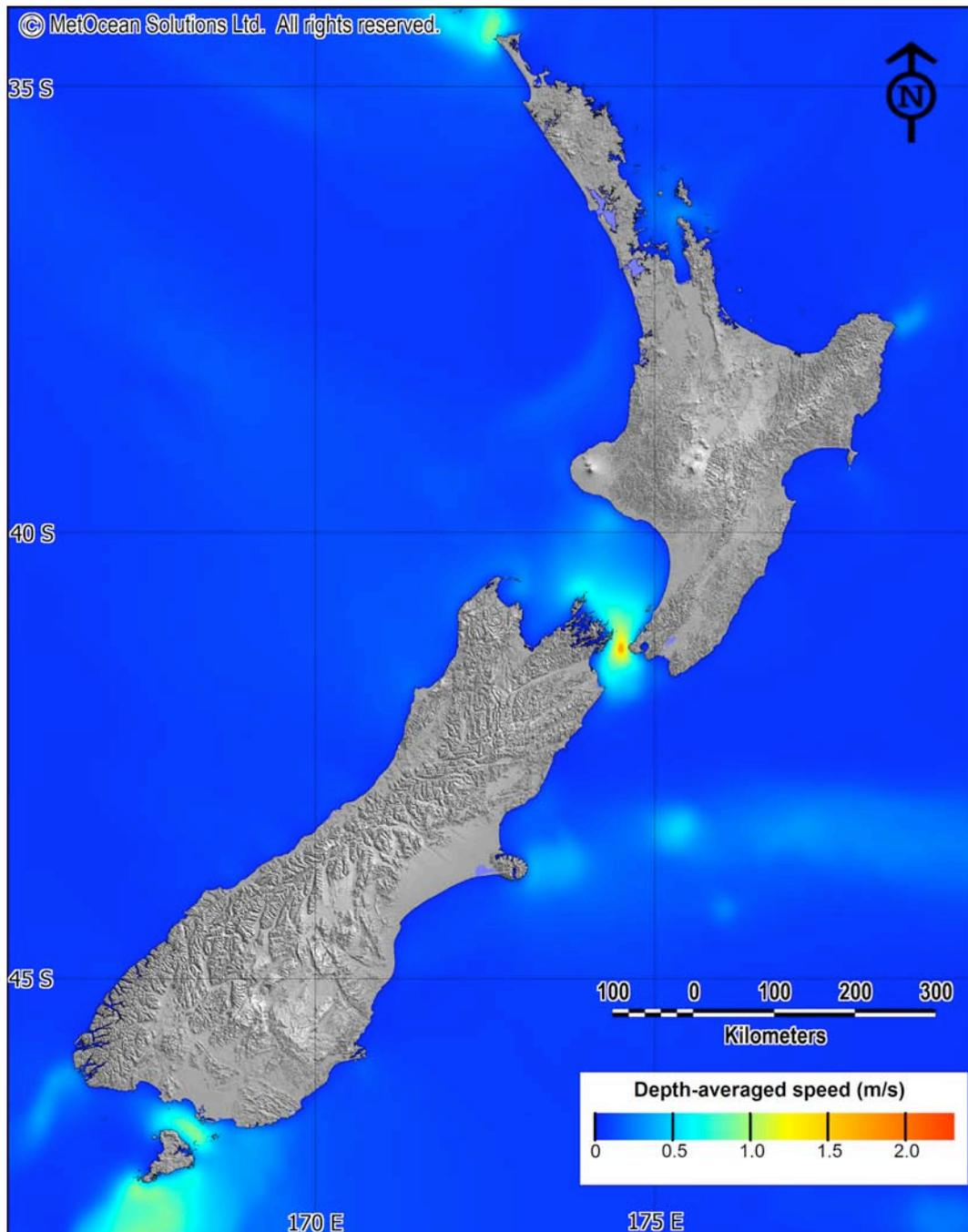
Figure 4: National Depth-averaged Tidal Current Speeds for Mean Spring Flows (in m/second)
