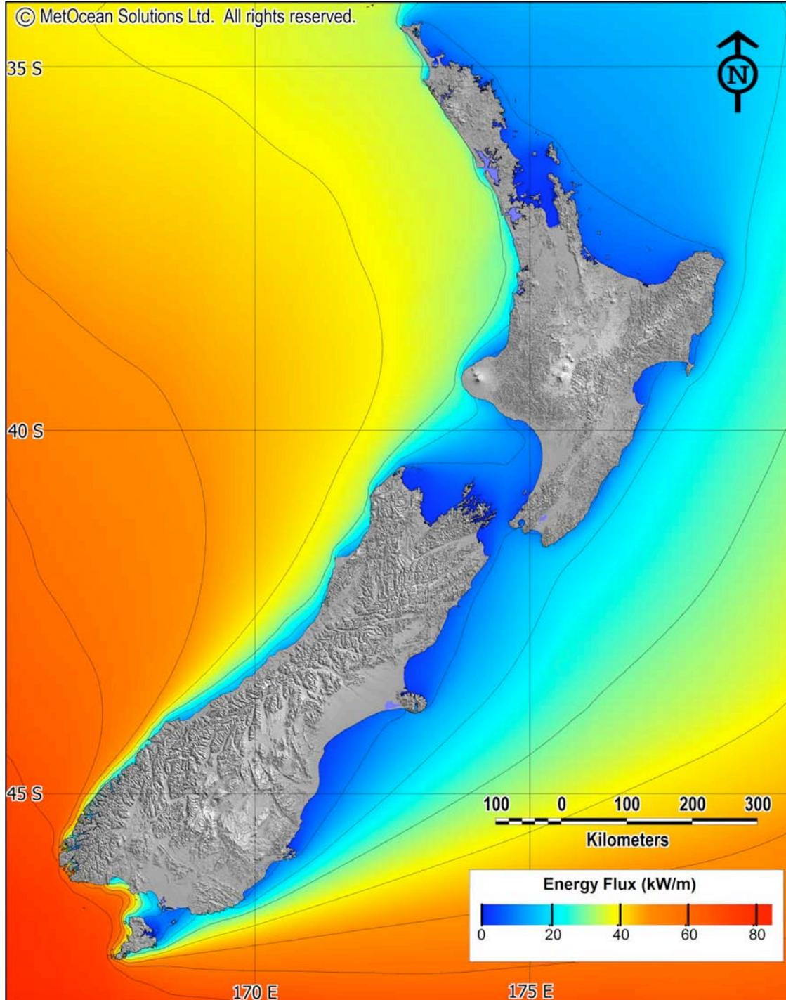
Figure 2: National Mean Spectral Wave Power in kW/m (1998 – 2007)
