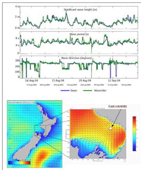
Figure 1: Validation of MSL wave hindcast with wave rider buoy data at Kupe gas field.
